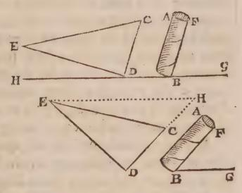
then the inclination of the revolutions in it, will be increased by the angle EDH, though these revolutions will still remain in a kind of ascent, so that water cannot bee turned through them.
